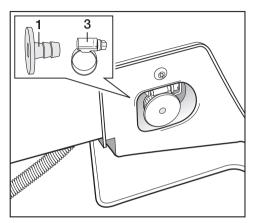
Remove the following from the back of the dryer at the bottom: Adapter 1 and hose clip 3 behind it.
